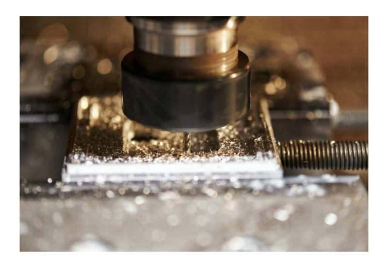
Above: the CNC milling from an aluminium solid. Previous page: the turning phase of a Neo plate.
